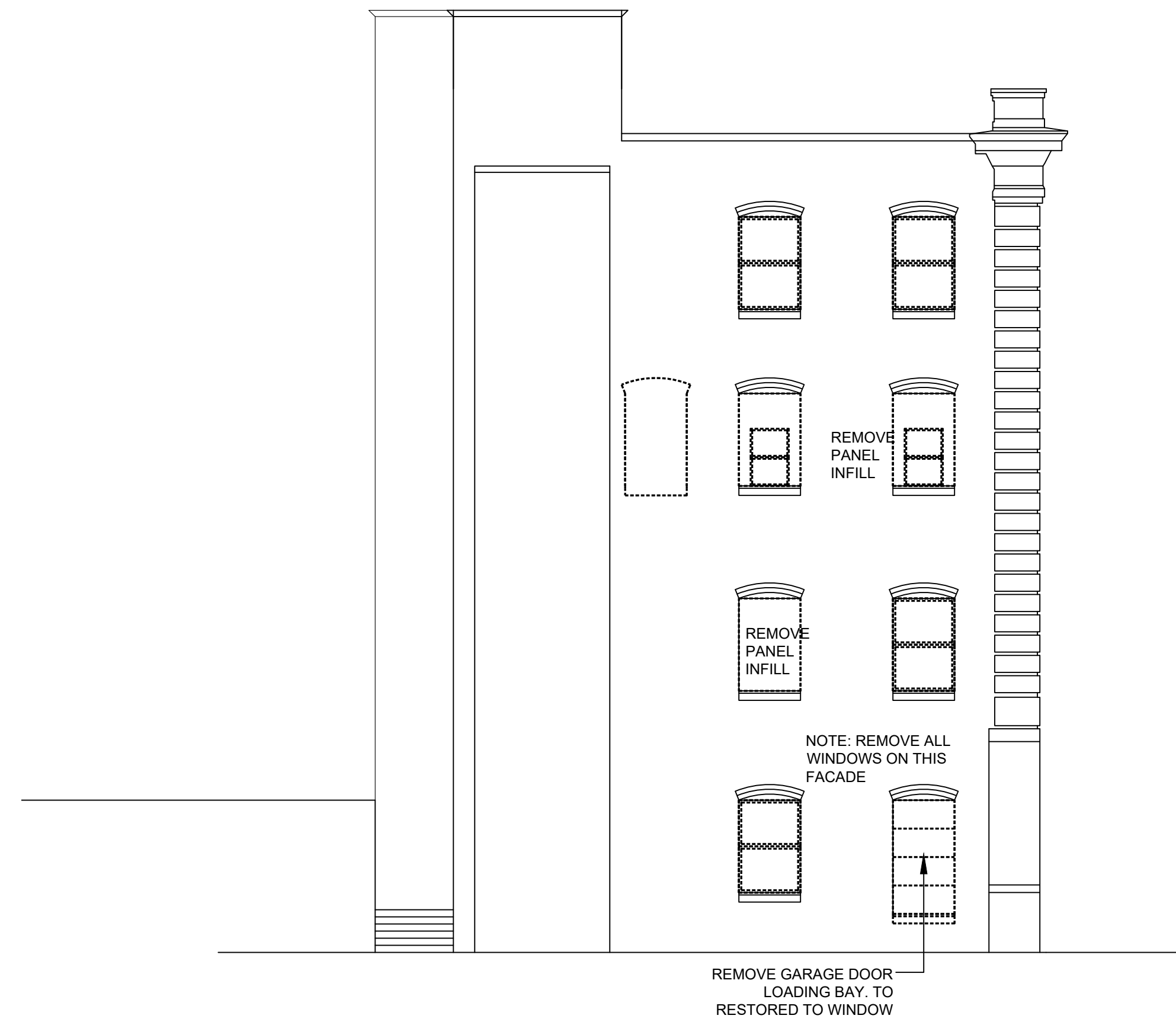
Existing North Elevation
