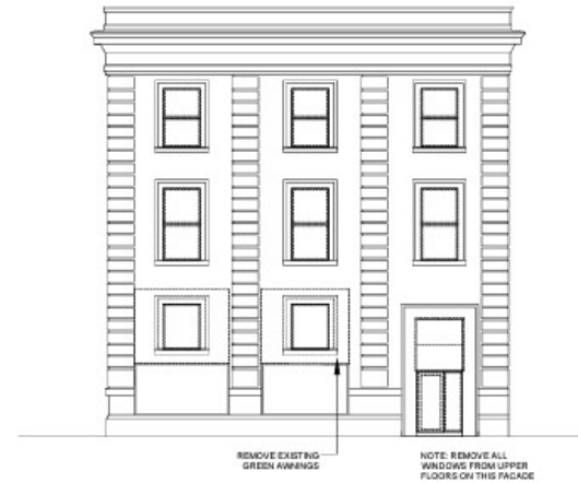
Existing South Elevation (Detroit) \frac{1}{8}'' = 1'-0''
