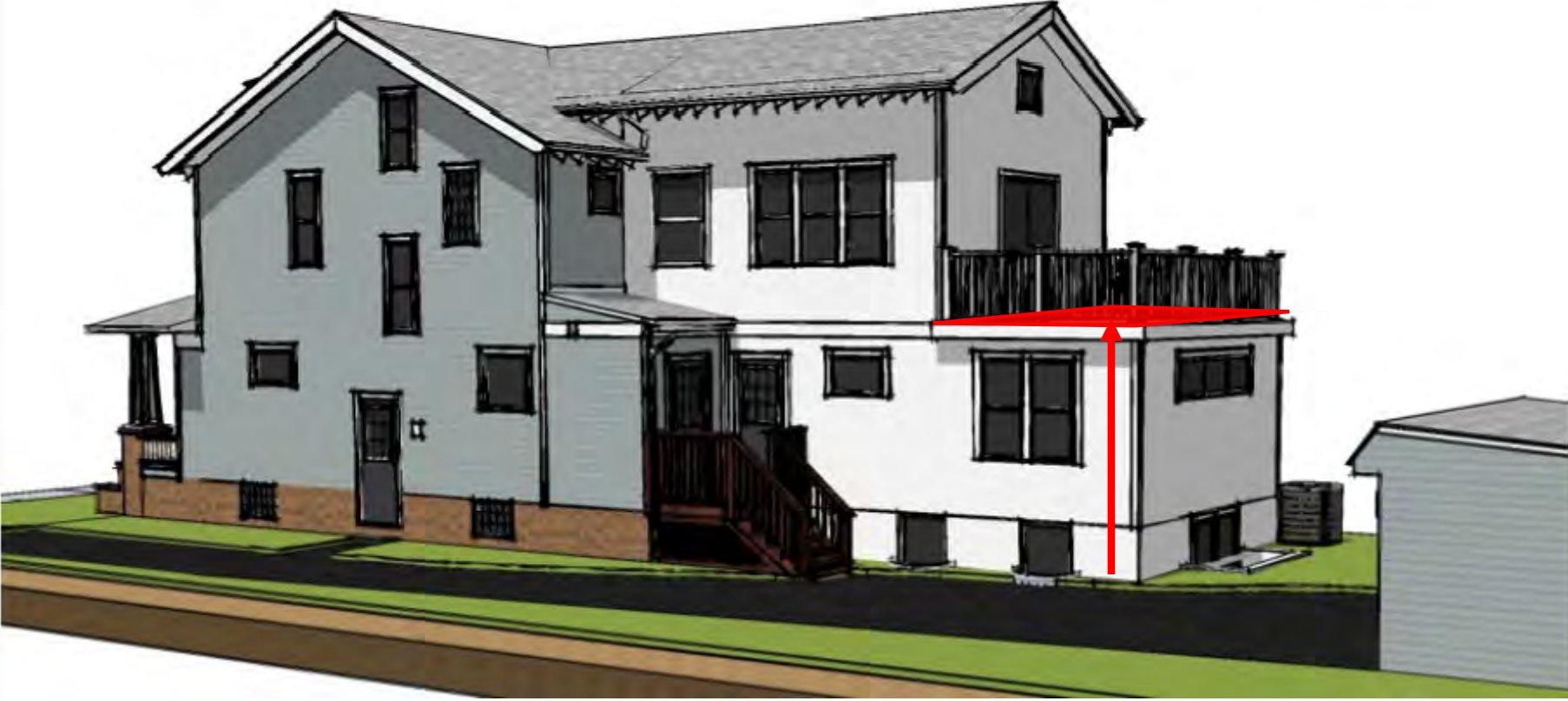
170 SQ. FT AREA - second floor unroofed patio deck 13' max - Height of existing second floor
