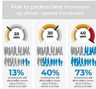
Source: Brian C. Tefft, 2013, AAA Foundation for Traffic Safety, Impact speed and a pedestrian's risk of severe injury or death . Figure 10. Likelihood of pedestrian death and severe injury due to speed
